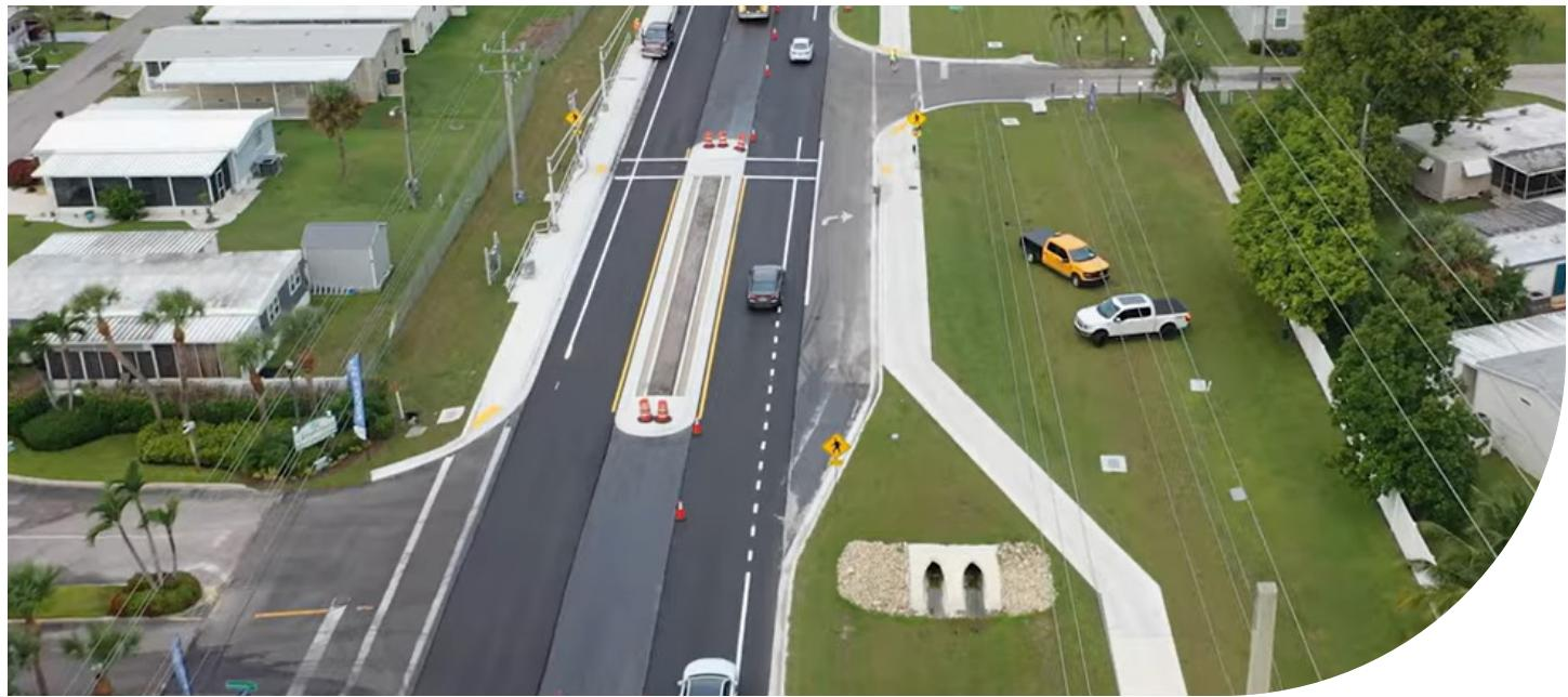
Lee County contracted with Stantec to design and permit the widening of Littleton Road from Corbett Road to US 41. Our team provided post-design services to assist the County's CEI. The 1.25-mile corridor consists of a 2-lane roadway with two water crossings at Yellow Fever Creek and the east branch of Yellow Fever Creek. Littleton Elementary School is immediately adjacent to the roadway.
