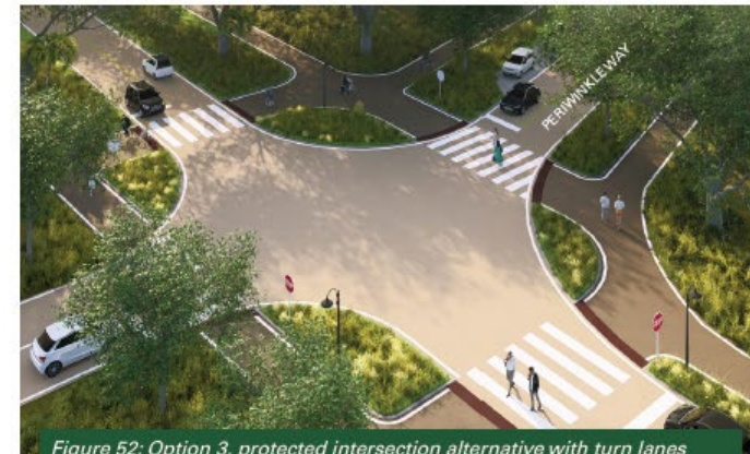
Figure 52: Option 3, protected intersection alternative with turn lanes removed and the overall roadway width reduced, decreasing impervious surface and increasing planting areas.
