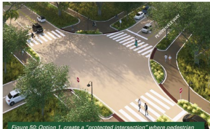
Figure 50: Option 1, create a "protected intersection" where pedestrian and cyclists are protected by a landscape buffer, and crosswalks reconfigured to reduce crossing distance.
