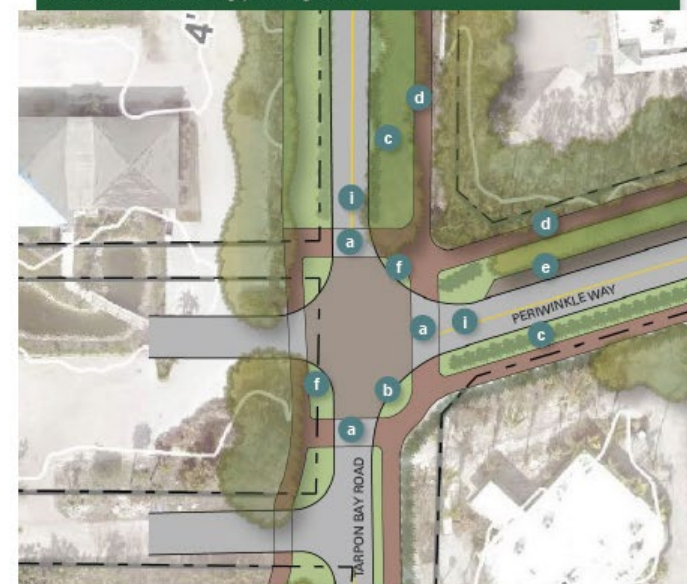
Figure 52: Option 3, protected intersection alternative with turn lanes removed and the overall roadway width reduced, decreasing impervious surface and increasing planting areas.
