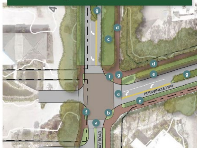
Figure 50: Option 1, create a "protected intersection" where pedestrian and cyclists are protected by a landscape buffer, and crosswalks reconfigured to reduce crossing distance.
