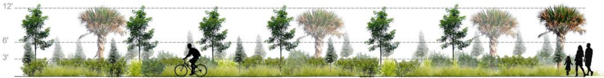
3A BUFFER ELEVATION 20' X 100' REDUCED LARGE TREE DENSITY (1 TREE / 200 SF) AT TIME OF PLANTING EX-3 SCALE: 1/4" = 1'
