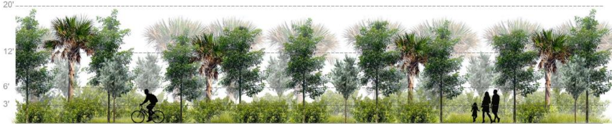
2B BUFFER PLANTING ELEVATION 20' X 100' WITH 15% REDUCTION FOR 100% NATIVE BUFFER SECTION AFTER 2-3 YEARS EX-2 SCALE: 1/4" = 1'
