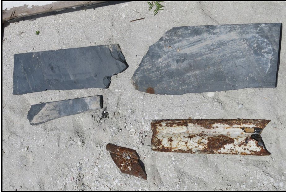
Photo 21. Three of the five recovered segments of slate from the Keepers' Quarters hearth (top) and two segments of the cast iron coal burning fireplace surround (bottom).
