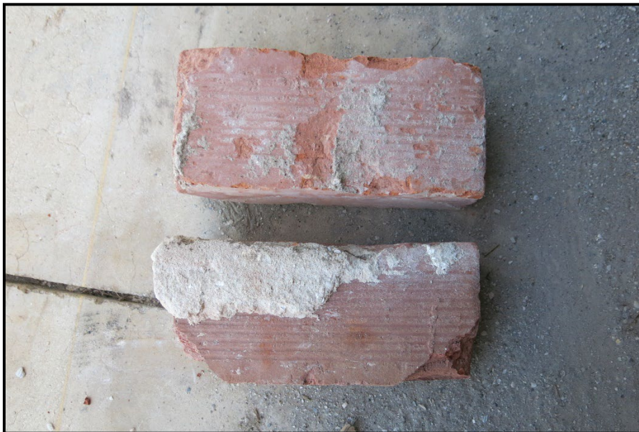
Photo 10. Examples of face brick (striated) identified within the relocated rubble pile. Intact segments of the cistern walls can be seen in Debris Pile – Group No. 2 below.
