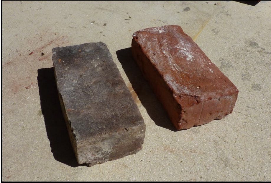
Photo 13. Examples of face brick (charred) (left) and face brick (plain) (right).
