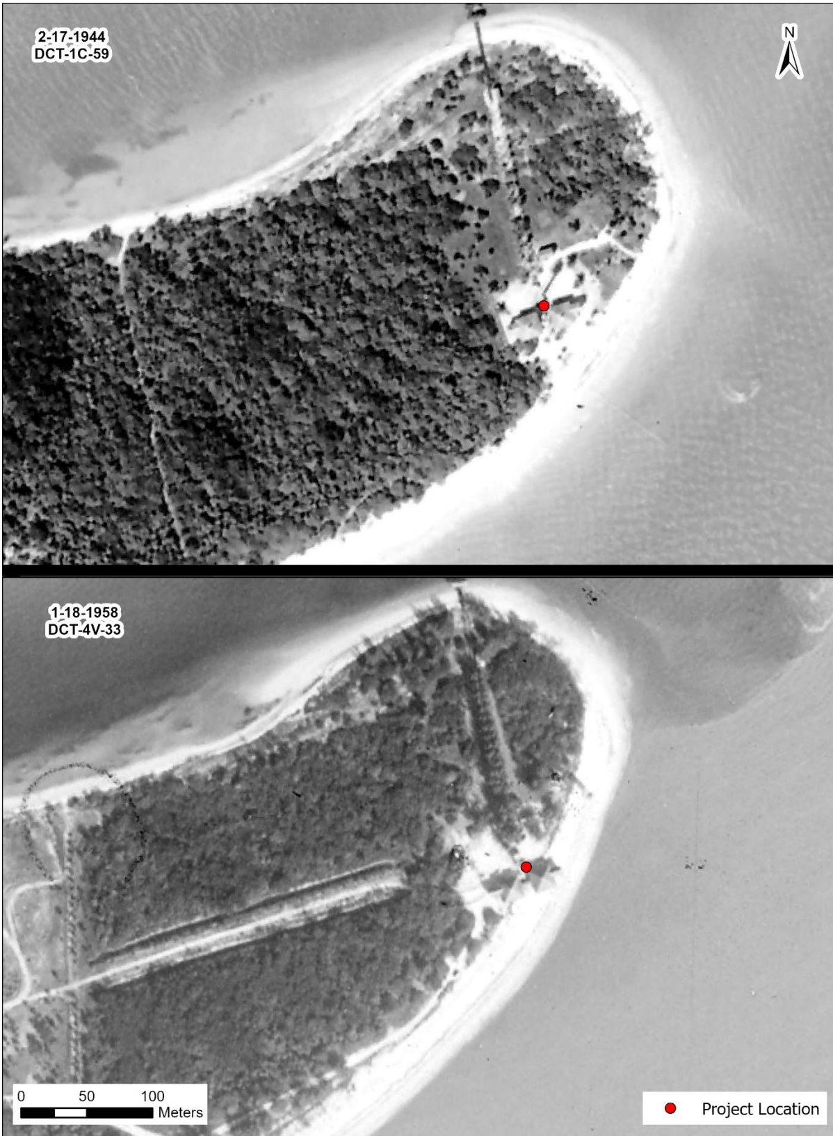
Figure 6. Historic aerial photographs showing significant beach erosion between 1944 and 1958.
