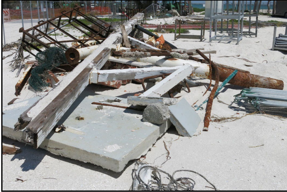
Photo 14. Wooden girder with intact metal support post and wooden brackets.
