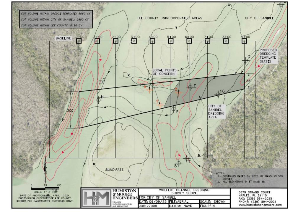
**Dinkins** Bayou Area 1 and Added Area 1 that is to be dredged with Wulfert Channel for access to the Henderson **Boat Ramp**
