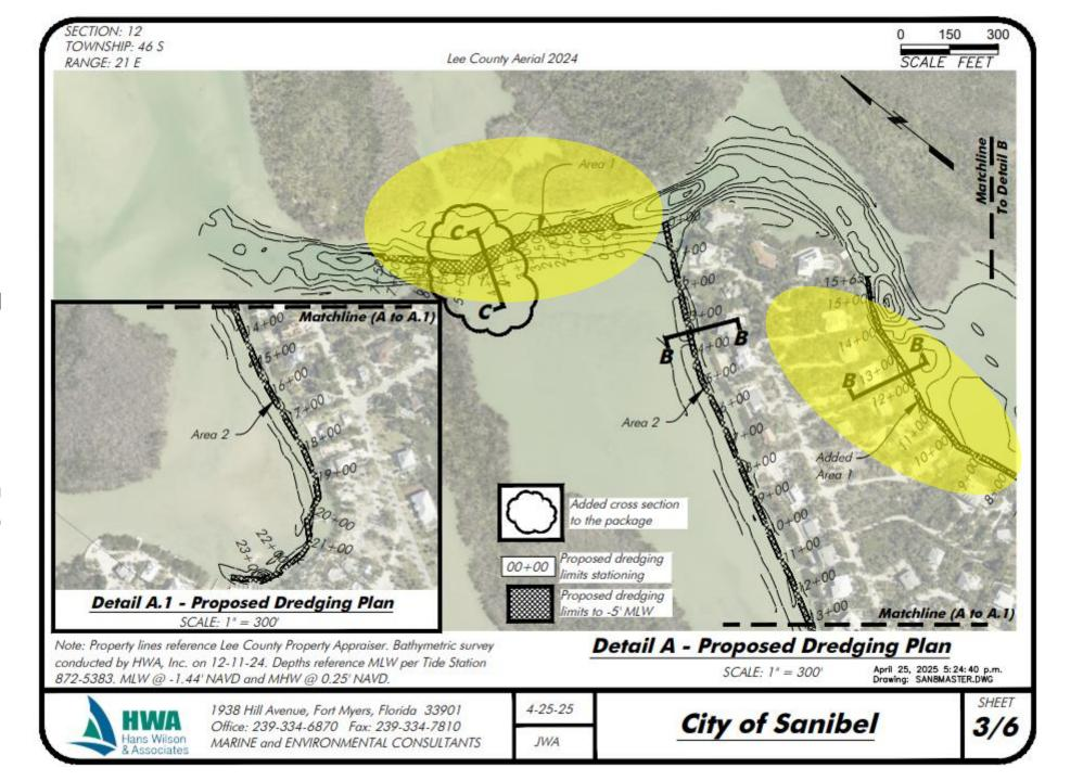
**Dinkins** Bayou Added Area 1 that is to be dredged with Wulfert Channel for access to the Henderson **Boat Ramp**
