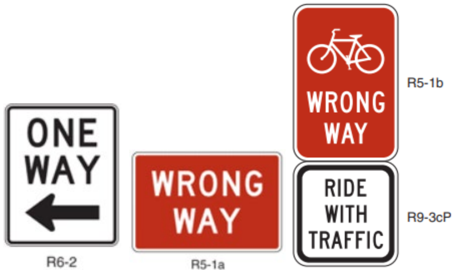
Figure 36. One Way and Wrong Way Signage 3
