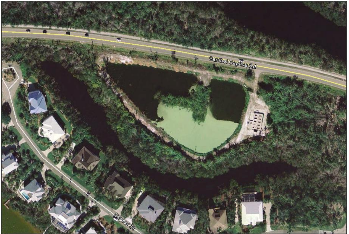
Figure 4. Imagery from 2005 showing the former percolation ponds and the adjacent Herons Landing stormwater pond. Perc pond surface area was approximately 61,200 square feet.
